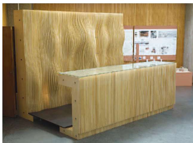
'Centenary Bar' at Sheffield University's School of Architecture, CNC machined Grade S/BB Birch Plywood with WISA-Hexagrip floor.
